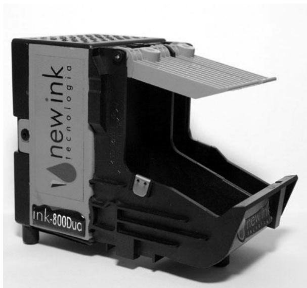
The 800 Dual Tester for HP 78 and 45 style Cartridges
